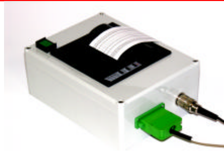
Connections for temperature and pressure probes and power supply
